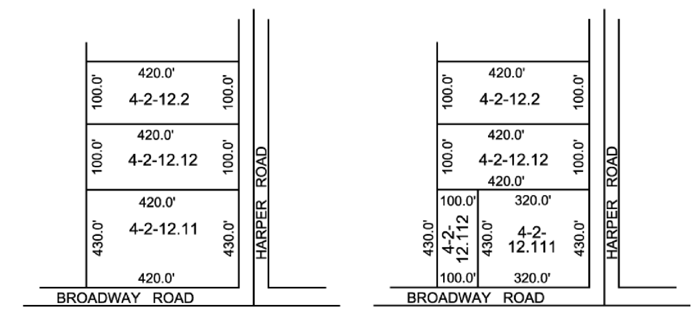
3. WHEN A PARCEL IS RESUBDIVIDED SUCH AS 4-2-12.1, THE PARCEL SOLD OFF BECOMES 4-2-12.12 AND THE RETAINED PORTION BECOMES 4-2-12.11.
