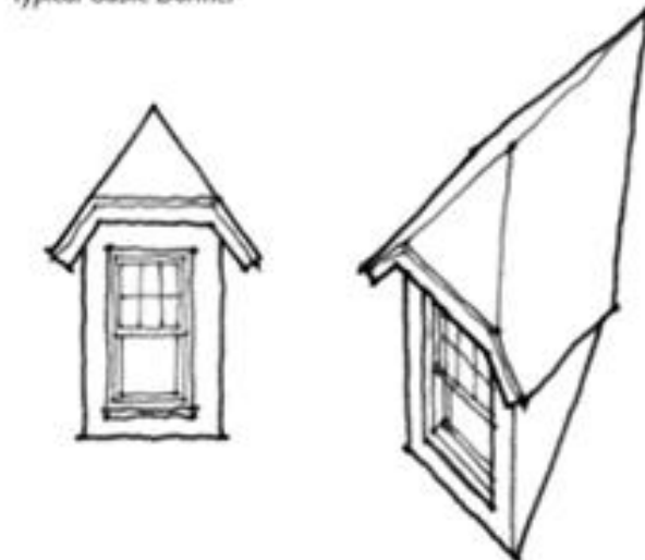
Typical Chamfered Dormer
