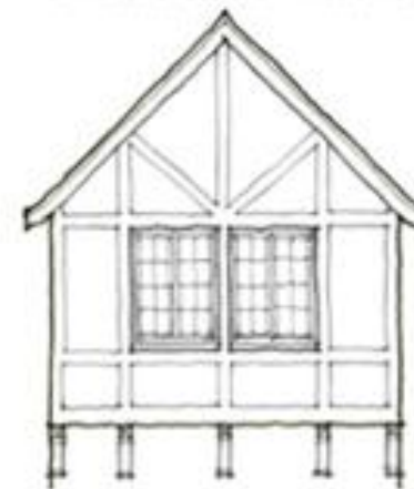
Typical Cantilevered Gable End
