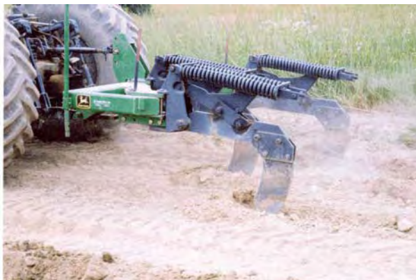
Fig. 10. An early pass with a 3-shank deep ripper penetrating only 8 inches into this worksite's severely compressed subsoil.
