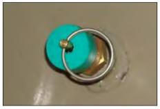
Figure 4. Automatic Pressure relief valve.
