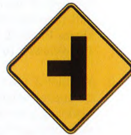
Intersection Warning Sign
