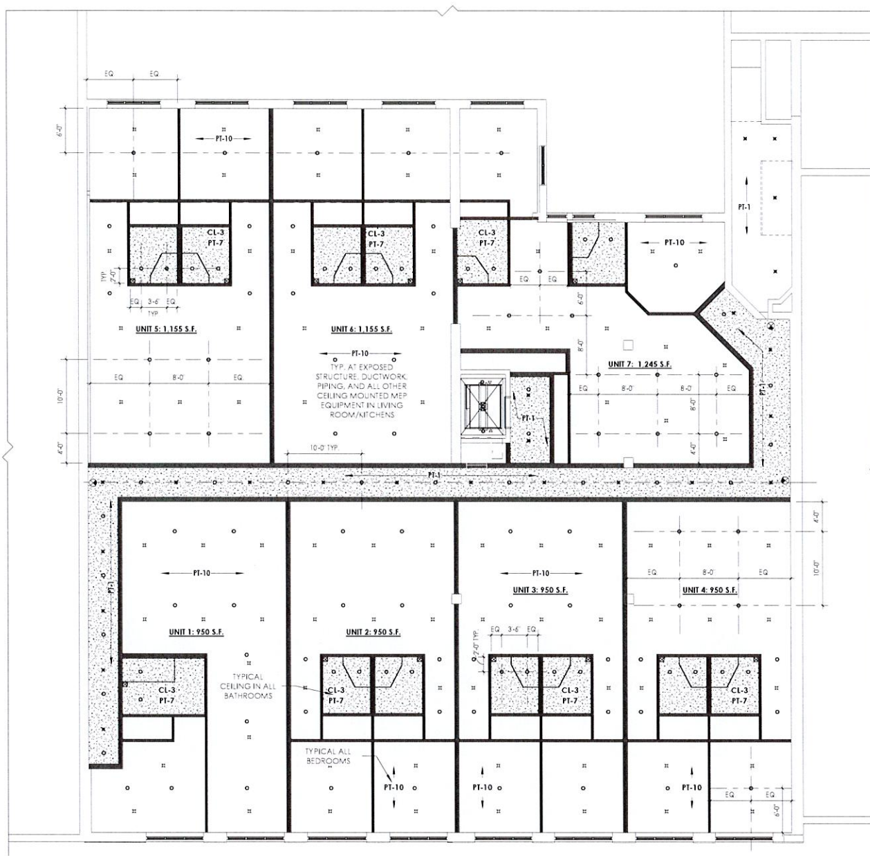
1 SECOND FLOOR REFLECTED CEILING PLAN TRUE NORTH A-602 1/8" = 1'-0"
