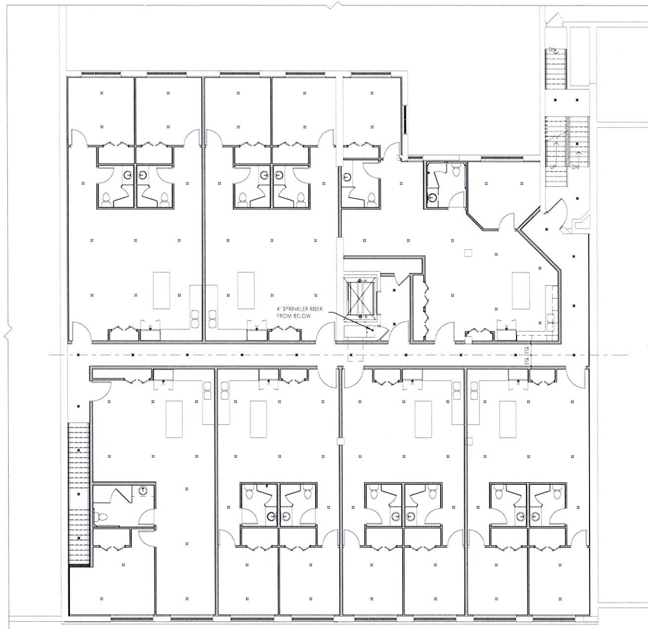
1 SECOND FLOOR SPRINKLER PLAN P-204 1/8" = 1'-0" TRUE NORTH
